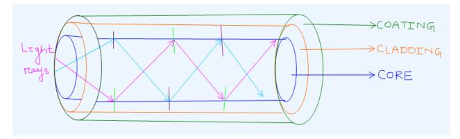
The light ray enters at one end of the fibre, undergoes multiple successive total internal reflections as the angle of incidence at the core cladding interface is always greater than the critical angle.
